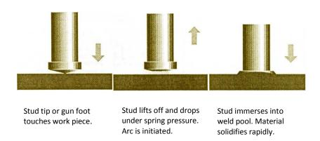
Note the final picture in the sequence above; in order for a weld to be good, it should have an even fillet completely around it. Any voids at all indicate a weakness in the weld zone that could only cause weld failure later. Also, the stud should appear to penetrate the parent material -- it should never appear to be 'sitting on top' of the weld.
